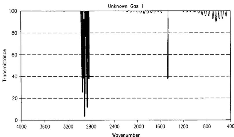
Fig. 4. The IR signature of the HHO gas made by the PdMA laboratory. When compared to the IR scans of Figs. 2 and 3, this scan shows that the HHO gas is not a mixture of H<sub>2</sub> and O<sub>2</sub> gases.
